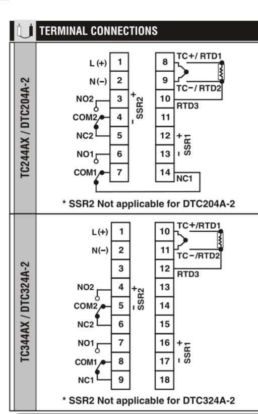
Use only the correct thermocouple wire or compensating cable from the probe to instrument terminals avoiding joints in the cable if possible. Failure to use the correct wire type will lead to inaccurate readings.
